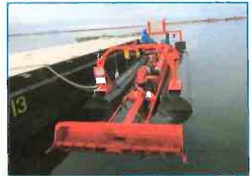
A Mud Cat MC 100E works on a channel maintenance project in the state of Washington.
