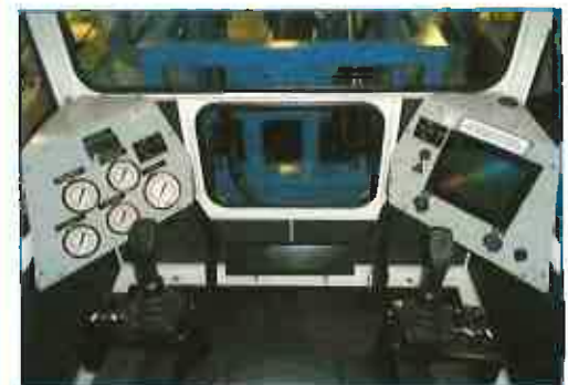
All Versi-Dredge® models come standard with joystick controls and oversized gauges for ease of operation.
