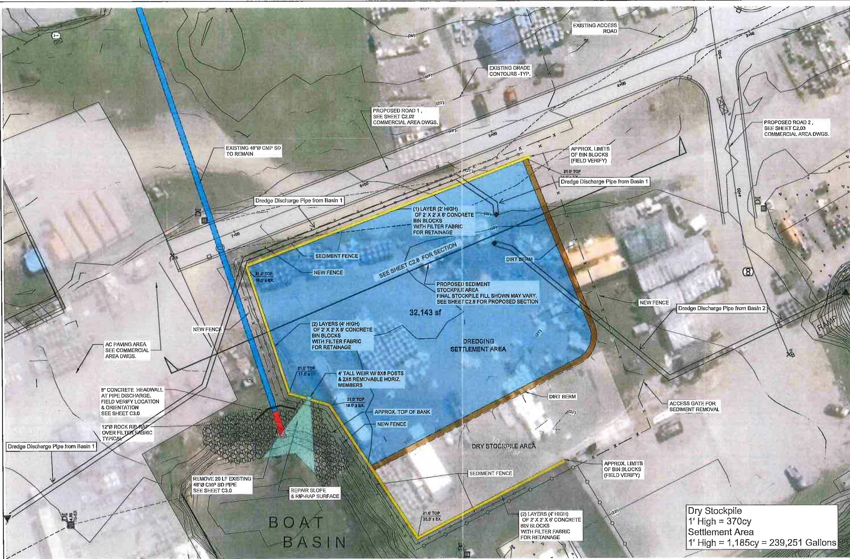
1 STOCKPILE GRADING PLAN SCALE 1" = 20'
